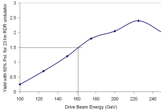
Figure 5: Yield associated with 60% polarization. 231m long RDR undulator with varying drive beam energy. Flux concentrator is used as OMD.
