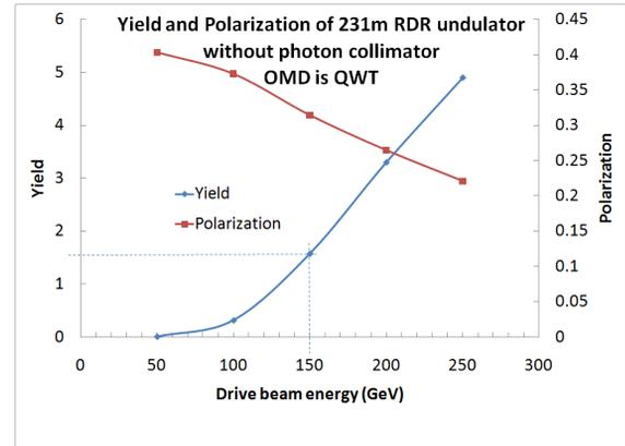
Figure 1: RDR undulator based positron source performance at different drive beam energy.
