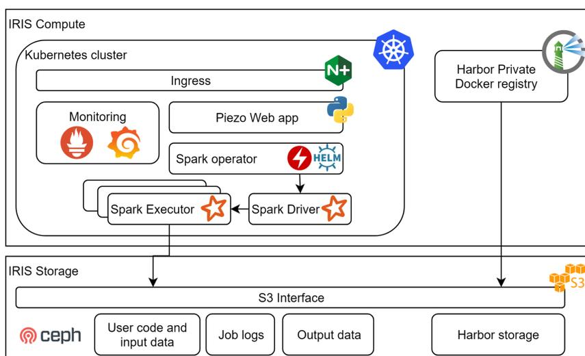
Figure 1: High-level Piezo component architecture
