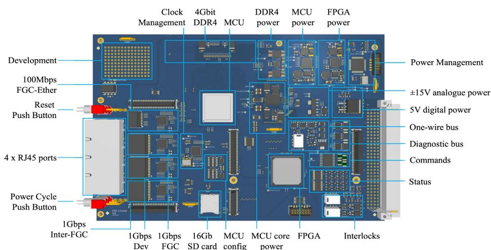
A hardware prototype FGC3.2 has been built, a diagram of which is shown on the left. The objective of the prototype is to validate the core design hardware choices for the FGC3.2, in particular:
