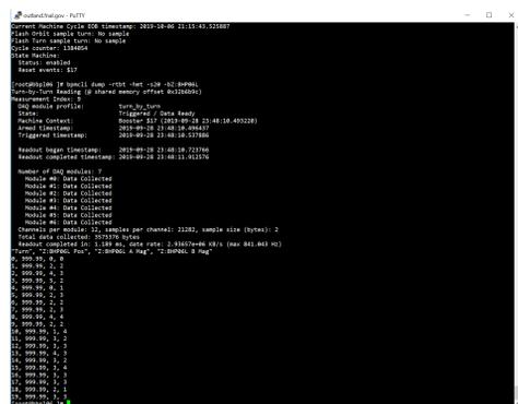
Turn-by-turn position measurement dump using the command line tool
