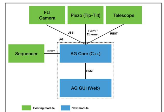
Figure 1: HARPS-N autoguider control architecture.
