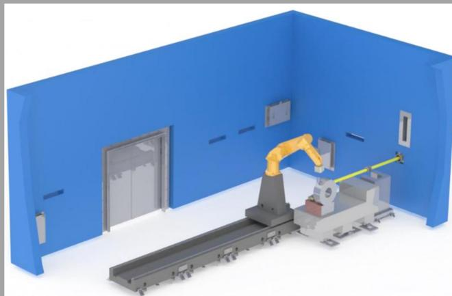
Robot used for X-ray coherent diffraction experiment at NANOSCOPIUM beamline
