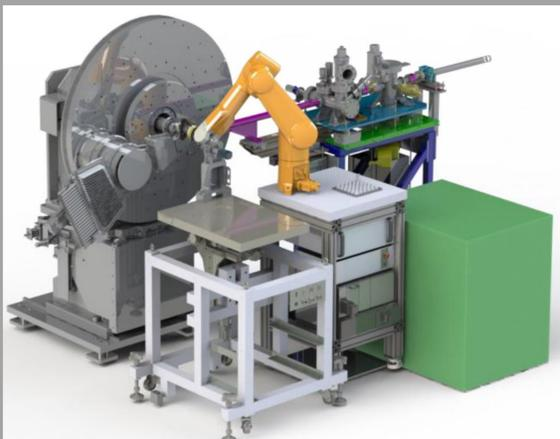
Robotic automation of powder diffraction experiments
