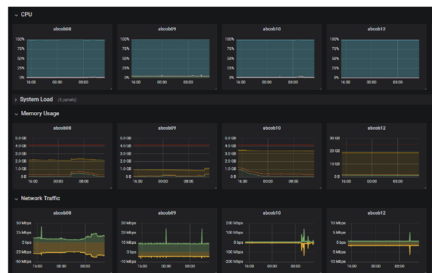
Figure 1: Grafana dashboard for computer performance metrics. The metrics are retrieved from Zabbix data storage.
