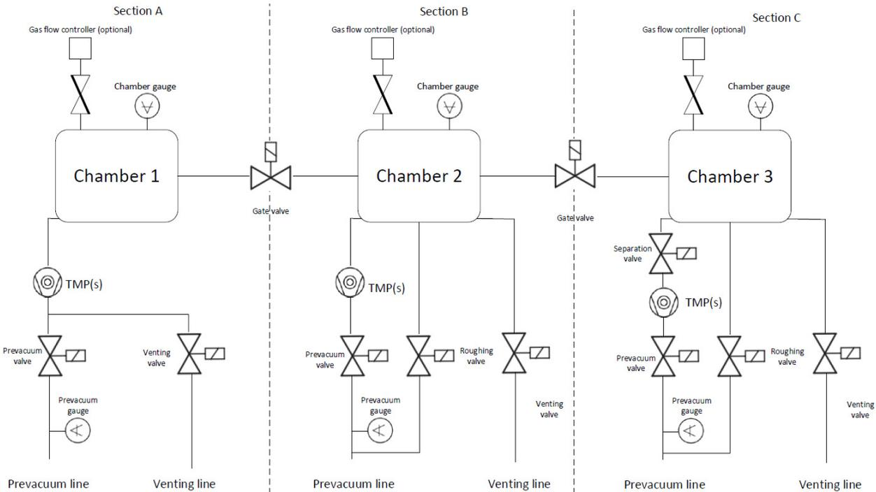
Figure 8: Most typical vacuum sections.
