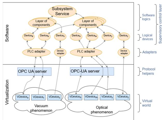
Figure 6: Layers of the Control system – virtualized devices.
