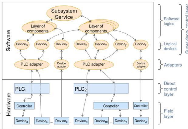
Figure 4: Layers of the Control system – low level device integration.
