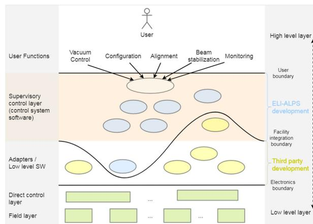
Figure 2: Control system scheme.
