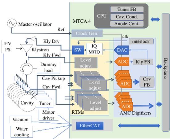
Figure 2: Block diagram of MTCA.4 system for Spring-8 LLRF.
