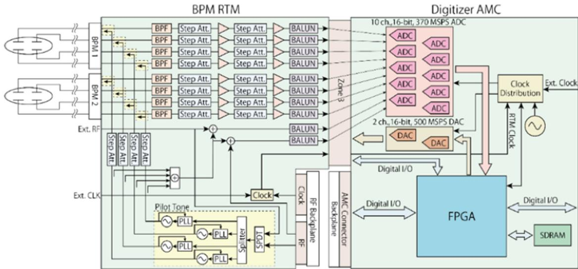
Figure 6: Block diagram of the BPM electronics.
