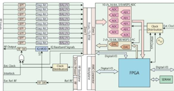
Figure 4: Block diagram of the digitizer AMC and a signal conditioning RTM.
