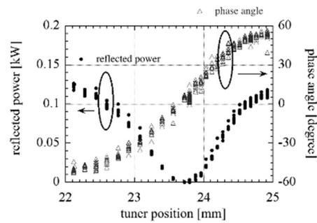
Figure 5: Reflected power from the cavity (filled circle) and the phase angle between the forward and the pickup signals (open triangle) as a function of the tuner position.
