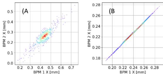
Figure 7: Scatter plots of beam positions from two BPMs. The SP BPM data with a 0.13 nC single bunch is plotted in (a) and the fast COD BPM data with a 30 mA stored current is shown in (b).
