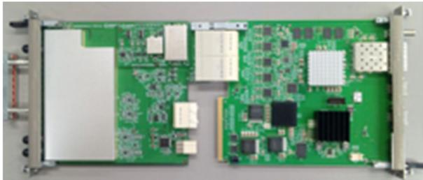
Figure 3: Photo of a digitizer AMC (right) and a signal conditioning RTM (left).
