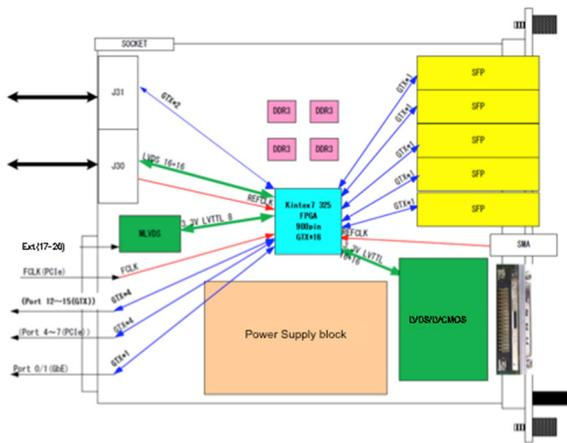
Figure 10: Block diagram of the trigger board.
