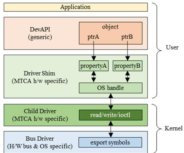
Figure 11: System structure of universal driver for MTCA.4 at SPring-8.
