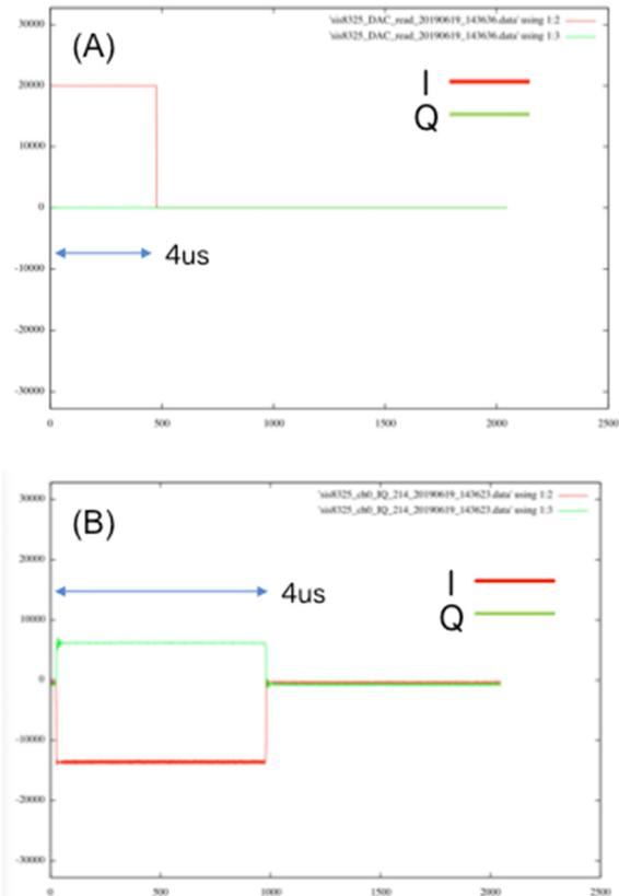
Figure 8: An output RF signal feed into RF input. An input waveform of vector modulator is shown in (a) and readout I/Q waveform is shown in (b).
