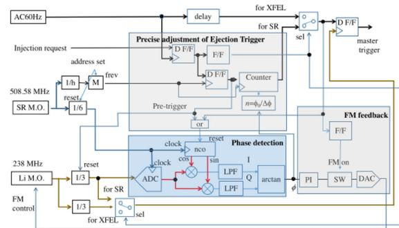
Figure 9: Block diagram of the synchronization system. The timing difference is measured at the phase detection section. The precise adjustment of the gun trigger is compensated by the frequency modulation.
