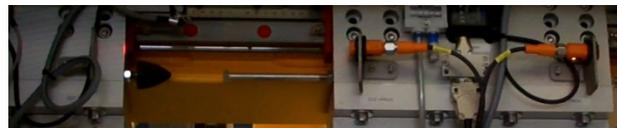
Figure 6: Proximity sensors, hard stop, and the soft dumper.
