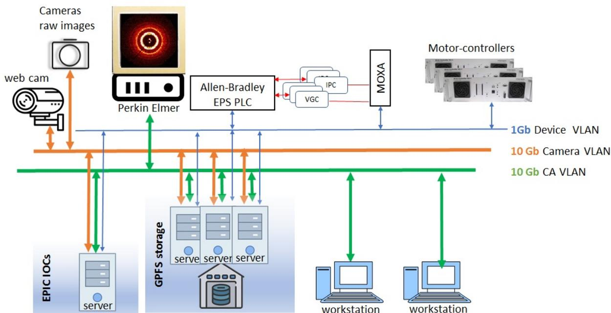
Figure 4: Beamline network has three dedicated Virtual LAN: low bandwidth device, raw camera data, and Channel Access (CA) client services.
