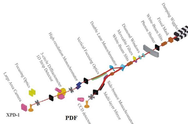
Figure 1: A schematic layout of the 28-ID optical configuration.
