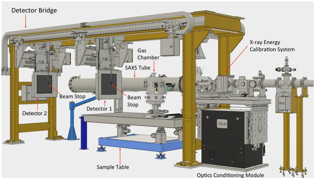
Figure 2: 3-D CAD layout of the OCM, Bridge, and the optics table.
