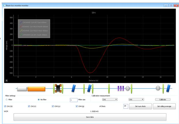
Figure 5: Response from Screen 05 inserted shown on user interface against a scaled diagram of the machine.
