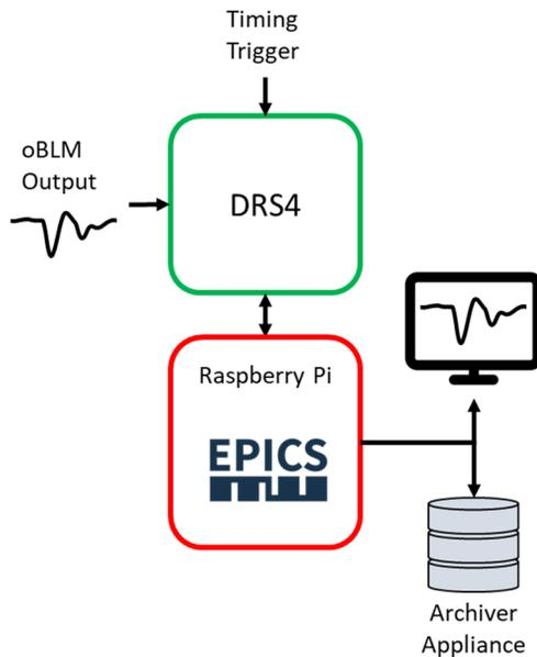
Figure 3: Data acquisition system.
