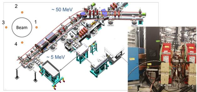
Figure 4: Quartz oBLM fibres laid over CLARA front end in North, South, East and West orientation.
