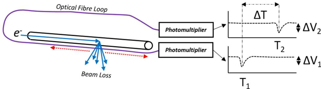
Figure 1: Principle of operation. Cherenkov radiation causes peaks in the voltage from a photo multiplier, the amplitude and delay of which is proportional to the magnitude and position of the loss respectively.
