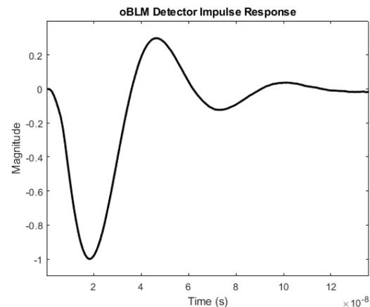
Figure 2: oBLM detector impulse response.
