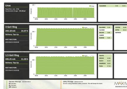
Figure 1: Screenshot of the MAX IV machine status web interface showing 11 open shutters during top-up mode operations of the 1.5 GeV and 3 GeV rings at 250 mA.
