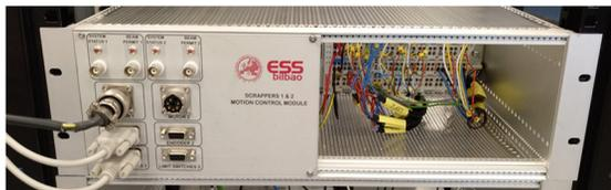
Figure 3: Scrapper pair, motion control Beckhoff rack.
