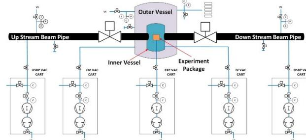
Figure 1: Beamline vacuum components.
