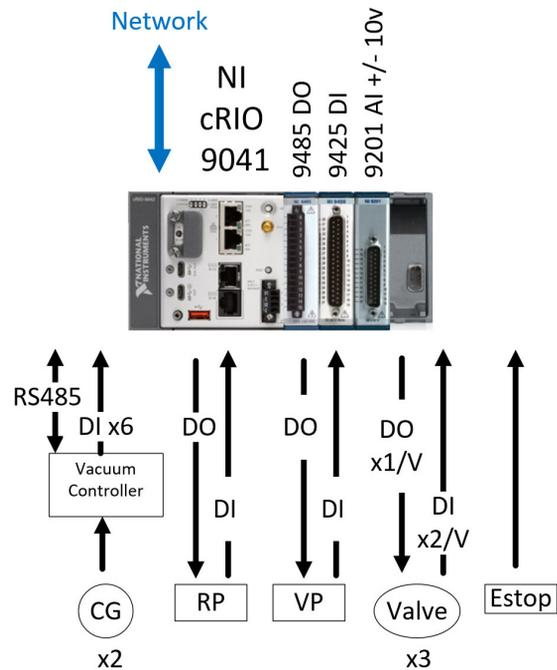
Figure 4: cRIO Vacuum Cart Control chassis.
