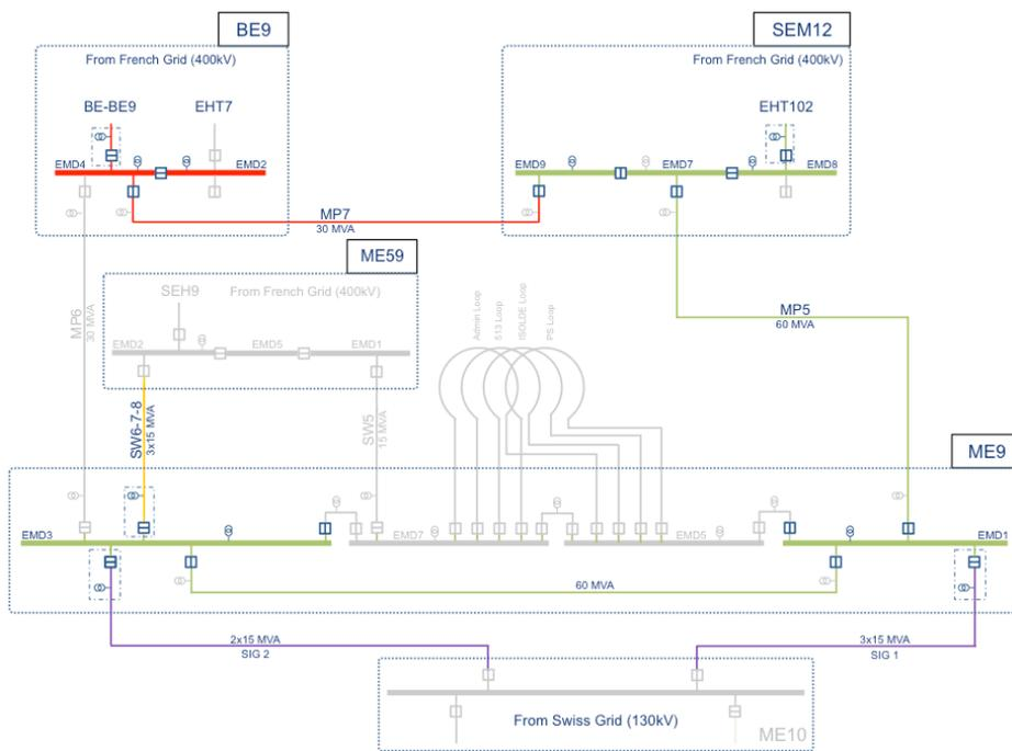
Figure 1: CERN 18 kV single line diagram representing the six sources capable of supplying the seven bus bars spread over the three main substations ME9, SEM12 and BE9. Breakers in bold are operated by the control system.
