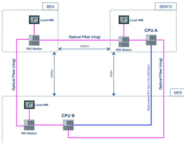
Figure 2: Auto Transfer control system PLC architecture.
