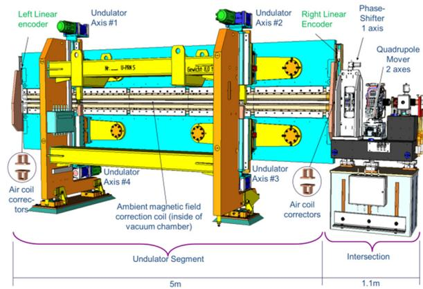
Figure 3: Undulator cell, consisting of undulator segment and intersection.
