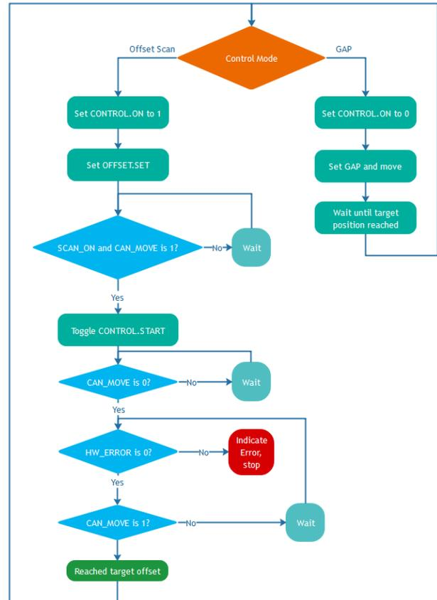
Figure 5: The flow chart of the undulator middle plane scan program.
