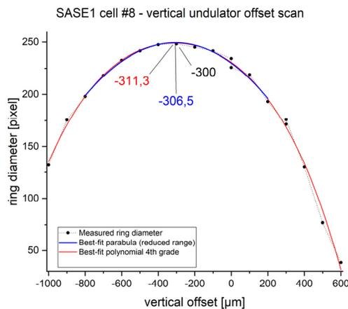
Figure 6: Ring radius versus vertical undulator offset.
