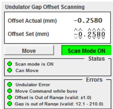
Figure 4: GUI for the manual control of the undulator middle plane.
