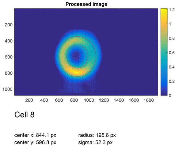
Figure 1: Example of online ring fitting, here for undulator segment 8 of SASE1.
