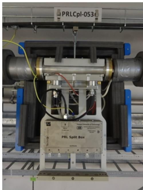
Figure 3: Tap Point interior (half of thermal insulation removed).
