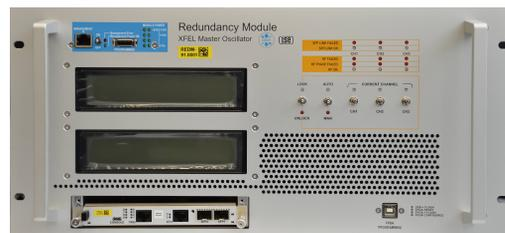
Figure 1: Photo of the XFEL Master Oscillator Redundancy Controller.
