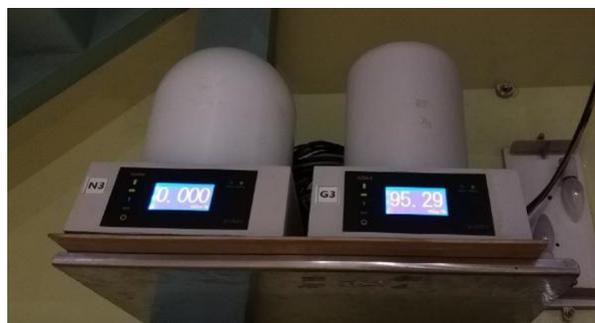
Figure 6: Neutron (n) and Gamma ray (c) detector.
