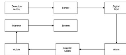
Figure 6: Diagram of smoke and gas detection.
