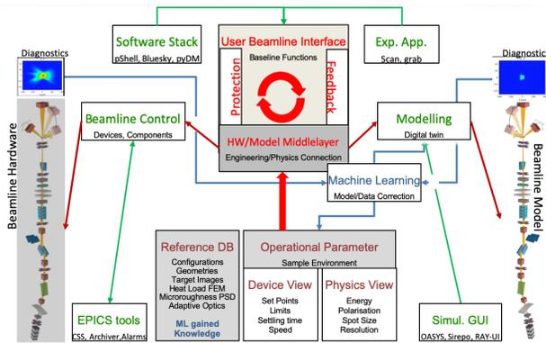
Figure 6: Sketch of the envisaged interplay of a high level user beamline control toolkit with configuration databases, device control, modelling and simulation software, diagnostics output and machine learning methods
