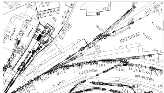
Figure 2: A small section of the experimental floor illustrates problems, that even arise for device naming. At BESSY sections of beamlines used in common split inside, outside or on both sides of the radiation protective wall. Dependent on the served instrument components in the common section change hardware representation, functionality and set point.
