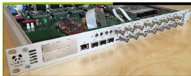
Figure 5: PandA provides a common encoder processing platform based on Zynq 7030, supports multiple encoder standards (incremental, SSI, BISS...) and delivers synchronous triggering and data capture capabilities [11].
