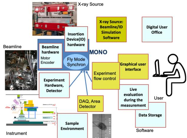
Figure 1: Sketch of the central role the multipurpose, generic software MONO (blue block) plays for the legacy experimental control infrastructure at BESSY
