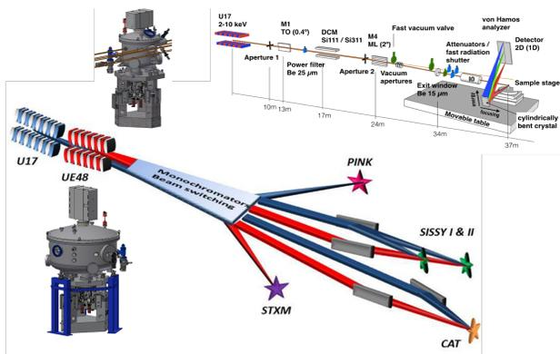
Figure 4: Two independent, canted undulators, two plane grating, one double crystal monochromator and multiple beamlines provide two color and polarisation combination x-ray capabilities to the Energy Materials In situ Lab (EMIL).
