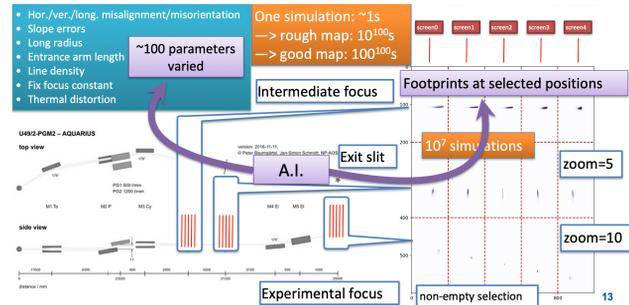
Figure 7: Process of model based generation of trained data for realistic beamline performance analysis.
