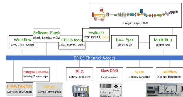
Figure 3: Plan for the refactoring, restructuring and reassembly of the experimental controls inventory. EPICS network representation has to be the unique integration layer for subsystems and software packages
