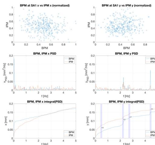
Figure 4: Example of using data from both sides: machine – here BPMs and experiment side – here the so called IPM (intensity-position monitor).
