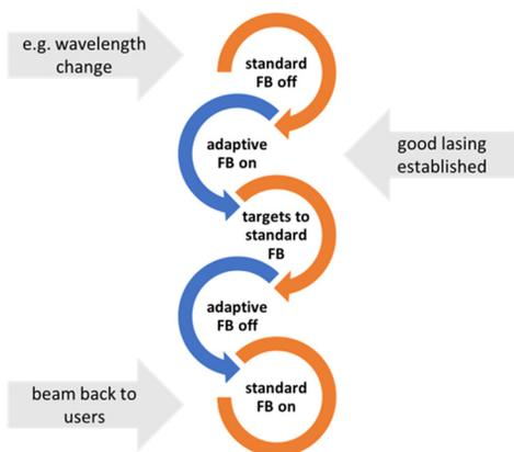
Figure 3: Typical sequence of interplay between using the standard and the adaptive orbit feedback.
