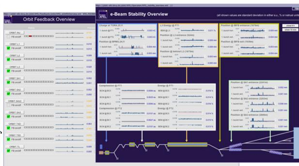
Figure 1: Some examples of using sparkline graphs for compact visualization of a bulk of parameters.
