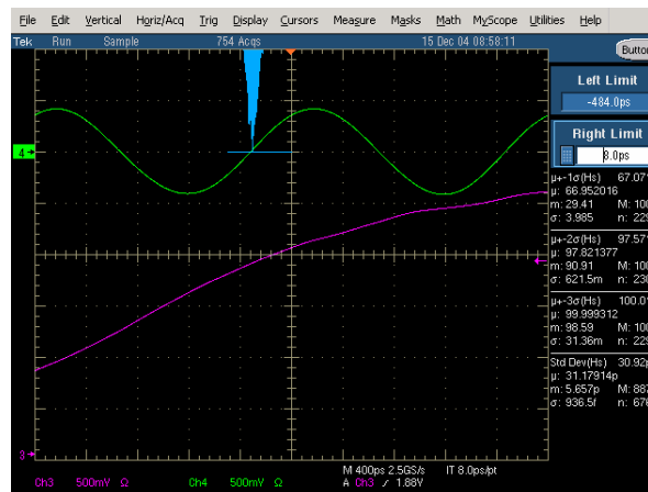
Figure 7 System jitter at 12.5Hz injection rate
