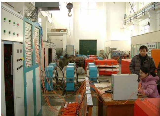
Figure 4 On-line test of Chopper power supply
