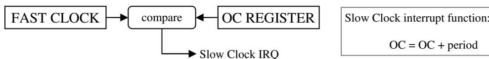
Figure 3: Trivial implementation of a slow clock using an Output Compare (OC) register
