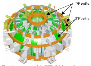
Fig.1 Arrangement of the KSTAR Magnet System
