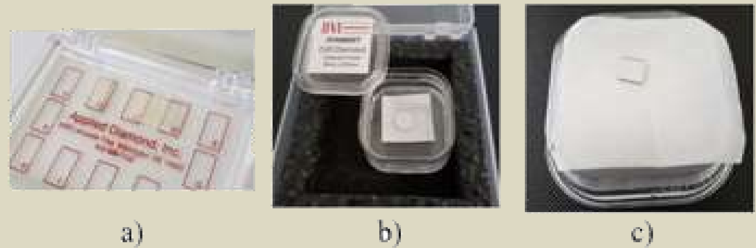
Figure 5: Diamond samples: a – CVD electronic grade sample from Applied Diamonds Inc., b – detector grade CVD diamond from II-VI, detector grade single crystal diamond from ElementSix.
