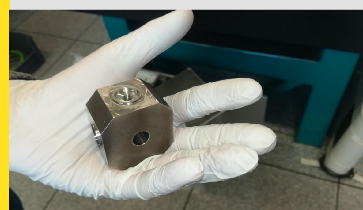
BPM after electrode welding
