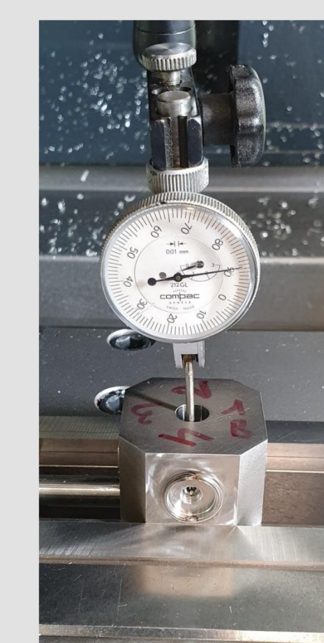
BPM block with the electrode positioning system before welding
