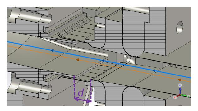
CST simulation for taper section and RF schileding foils:  $k \approx 2 \times 10^{14} \text{ V/C/m}$ .
