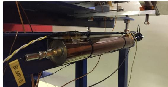
Figure 1: A gas-based BLM installed under the magnet.
