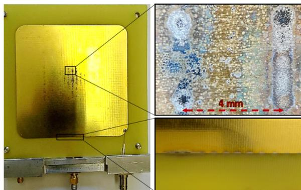
Figure 9: Photo of plane electrodes of proportional chamber subjected to degradation.
