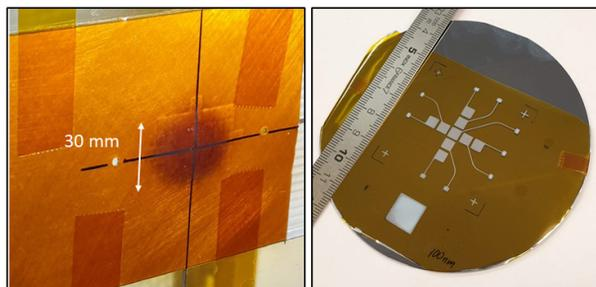
Figure 1: On the left, old BPM device, consisting of a PCB patterned with a matrix of sensing pads from copper in multiple layers. The footprint of the beam can be observed. On the right, the new BPM device, consisting of aluminum sputtered on polyimide substrate.
