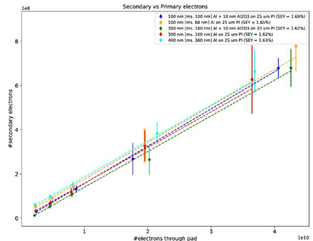
Figure 5: SEY measured for the different BPMs tested at the CLEAR facility.
