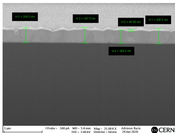
Figure 6: Focused Ion Beam (FIB) analysis on a 400 nm samples, confirming an average thickness of 380 nm.
