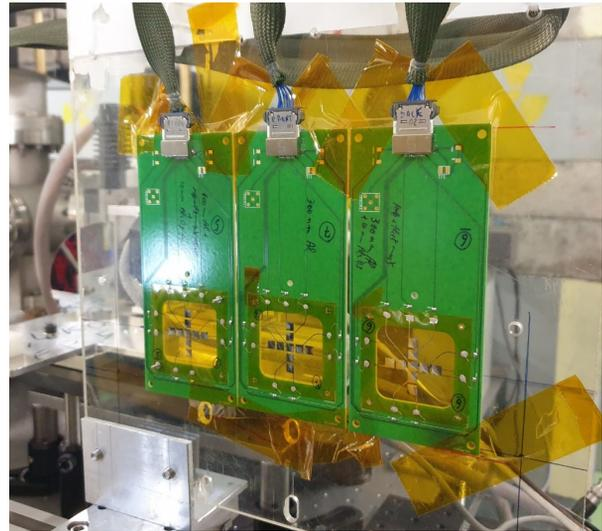
Figure 4: Experimental setup for the CLEAR irradiation tests. The BPMs were mounted on dedicated PCBs and attached to a Plexiglas support. The support, in turn, was mounted to a motorized stage which allowed positioning the devices under the beam spot.
