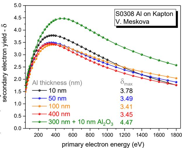
Figure 3: SEY spectra of metallized Kapton samples with different metal layer thickness. Tests were performed in a vacuum enclosure and bombardment by low energy electrons.
