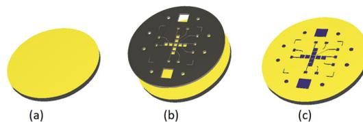
Figure 2: Shadow mask deposition technique. (a) Thin polyimide film on a silicon wafer support. (b) Shadow mask put on the top on the polyimide. (c) BPM design patterned on the top on polyimide after aluminium sputtering process.
