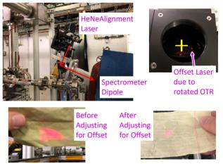
Figure 5: Alignment of the transport line is via a HeNe laser injected through a viewport before the spectrometer magnet. The before and after pictures show the distortion induced by the rotated OTR screen. The yellow cross is the ideal laser position.
