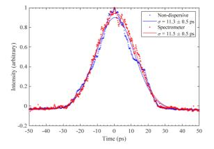
Figure 7: Projections of streak camera images from both the new spectrometer line and the upstream non-dispersive line.
