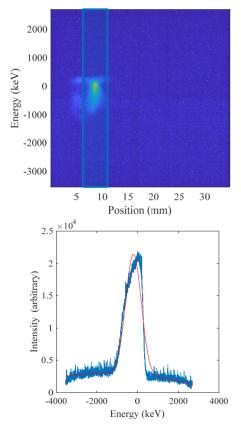
Figure 9: Top) Spectrometer camera image of beam with 15-degree rf phase offset. Bottom) The energy spread projection within the boxed region of interest and a gaussian fit with sigma of 383 KeV.
