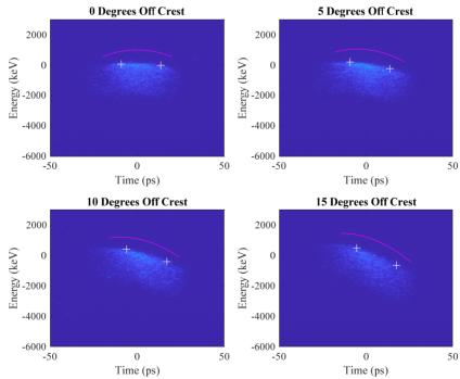
Figure 8: Streak camera images for four phase offsets of the CC1 accelerating gradient. The white crosses are the points used to determine the slope induced by the rf phase offset, and the red curves are the expected energy curve given the calibration from the points. For reference, a micropulse rms length of 11.5 ps corresponds to 6.2 degrees.
