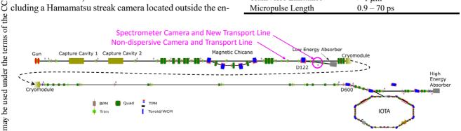
Figure 1: Layout of the FAST facility. D122 is the spectrometer magnet, after which is the OTR source for the new optical transport line.
