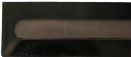
Figure 2: MMD 1024, 1024 strips with a pitch of 60 \mu\text{m} for heavy ions registration in mass spectrometry.
