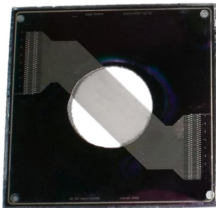
Figure 4: MMD64, 64 strips with a step of 100 \mu\text{m} – for XY-positioning and profiling of mini- and micro-beams of charged particles and X-ray radiation.
