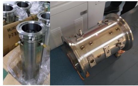
Figure 5: Stripline BPM designed for LINAC (left) and shoe-box BPM for RTBT (right).
