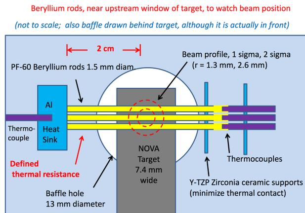
Figure 3: Schematic of the Hylen Device.
