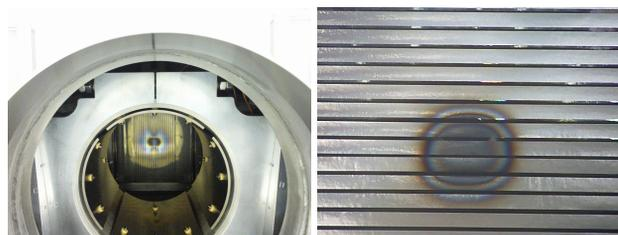
Figure 4: A photograph of the SSEM19 downstream (upstream) foil after  $2.3 \times 10^{21}$  ( $3.2 \times 10^{21}$ ) incident protons is shown on the left (right).
