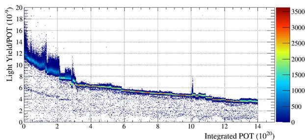
Figure 5: OTR yield decrease over  $\sim 1.4 \times 10^{21}$  incident protons.
