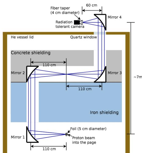
Figure 2: Schematic of the J-PARC extraction beamline Optical Transition Radiation monitor.
