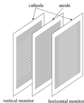
Figure 1: J-PARC neutrino extraction beamline Segmented Secondary Emission Monitor design.
