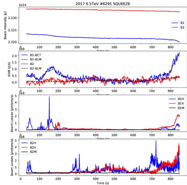
Figure 11: Example of beam loss decomposition. Stored beam current as function of time (top), beam loss rate as a function of time (middle), beam loss rate for each plane as function of time (bottom).
