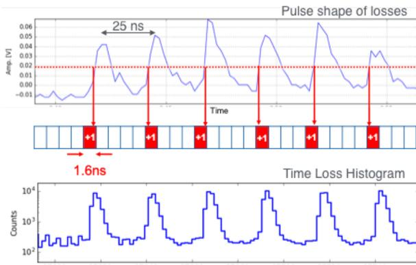
Figure 5: Raw amplitude signal as a function of time (top). Resulting histogram with bins of 1.6 ns with the accumulated counts on the y-axis (bottom). Image credit: Ch.Xu.
