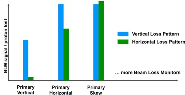
Figure 9: Diagram showing the signal of several BLM detector for different loss patterns.
