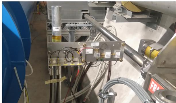
Figure 4: Picture of one Diamond BLM in the LHC tunnel in one of the collimation areas. Image credit: J.Kral.
