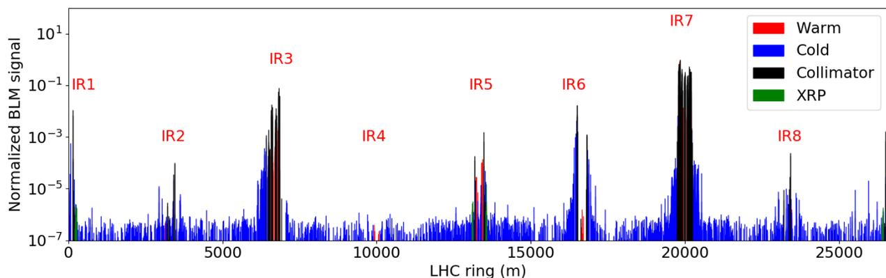
Figure 2: Normalized beam losses measured with ionization chambers along the LHC ring, each line corresponds to the measurement of one IC BLM.
