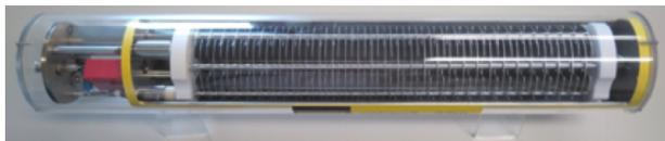
Figure 3: Picture of one IC BLM detector with the cylinder open in order to show the interior.
