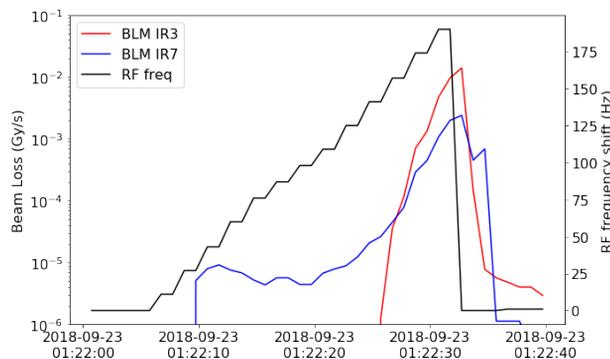
Figure 13: Distribution of beam losses after a primary collimator in IR3 (red) and in IR7 (blue) together with the change of RF frequency (black) as function of time.
