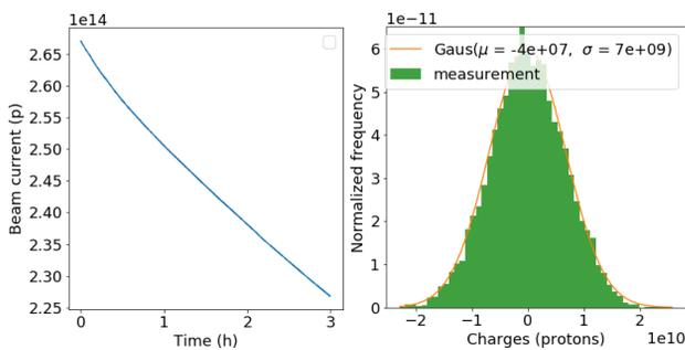
Figure 6: Beam current measurement at LHC during stable beams (left) and statistical noise analysis of the measured signal (b).
