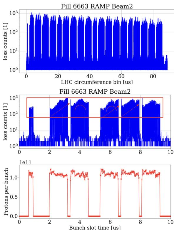
Figure 12: Loss count distribution from dBLM detectors as a function of bunch location (top) with its zoom (middle). Number of protons per bunch as a function of the zoomed area (bottom). Image credit: A.Gorzawski.
