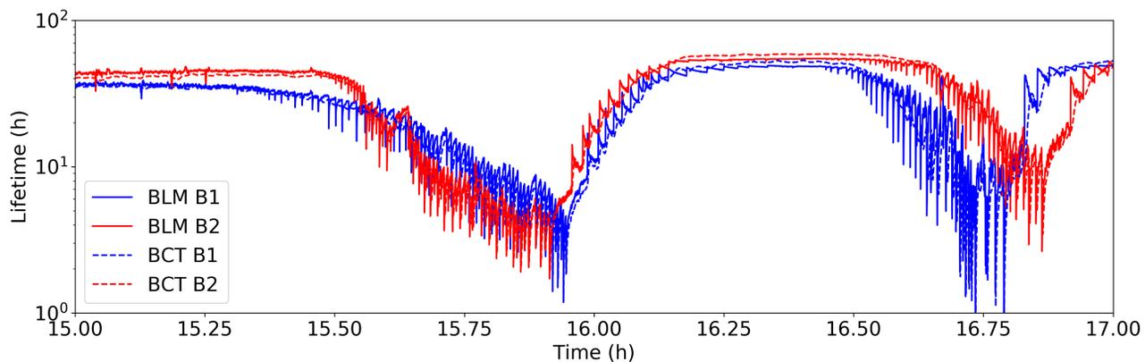
Figure 7: Beam lifetime during beam halo scraping at the LHC reconstructed with the combination of 4 BLM detectors per beam (solid lines) and the BCT (dashed lines).
