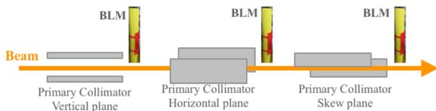
Figure 8: Diagram showing the position and orientation of the primary collimators in IR7.
