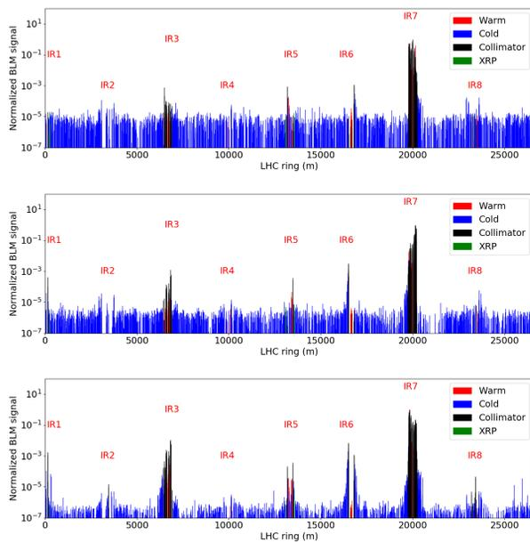
Figure 10: Loss maps for three different configurations: Beam 1 vertical losses (top), Beam 2 horizontal losses (middle) and both beams off-momentum losses (bottom).
