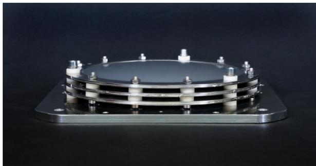
Figure 1: SEM detector developed for FAIR.
