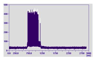
Figure 6: SiPM response, 400 bunches @ 1MHz rep. rate + 1 bunch, scintillator, bias +27V.
