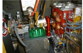
Figure 2: BLMs in undulator intersection.
