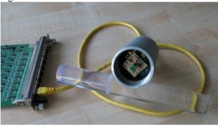
Figure 10: RTM and BLM with SiPM readout (prototype).
