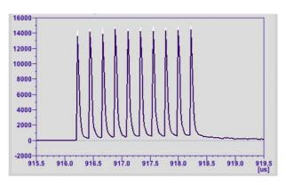
Figure 7: SiPM response, 10 bunches @ 4.5 MHz rep. rate, cherenkov, bias +29V.
