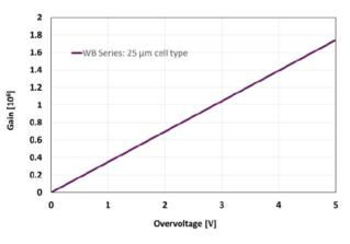
Figure 4: SiPM gain versus bias voltage [3].
