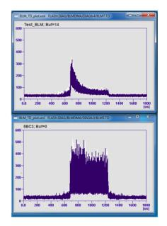
Figure 5: SiPM (top) vs. PMT (down); Darkcurrent signal over pulstrain; SiPM bias voltage drops due to too less bias current.
