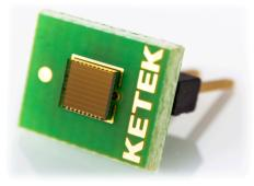
Figure 3: PM3325-WB-D0 from KETEK on PCB with pins.
