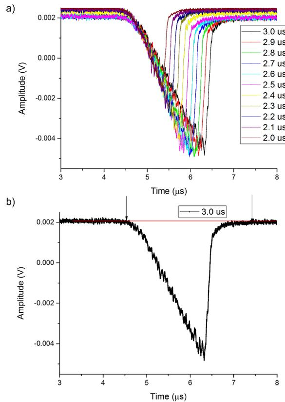
Figure 3: oBLMs signals from one channel for different RF pulses length is presented by different colours on top graph. The RF pulse was varied within 3.0  $\mu$ s to 2.0  $\mu$ s. From graph a) it can be seen that the oBLMs signal follows the shape of the pulse and its length can be reconstructed from the oBLM signal. Graph b) shows the oBLM signal which was obtained for 3.0  $\mu$ s pulse.
