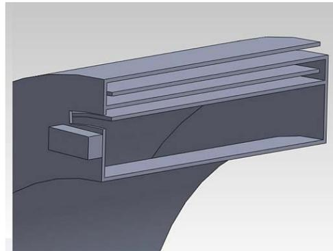
Figure 5: Alternative shielding geometry with axial meanders.
