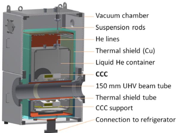
Figure 9: Design of the cryostat for the FAIR CCC.
