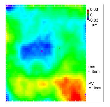
Evaluation of the wave front by its root-mean-square rms distribution and the maximal peak-valley PV difference.
