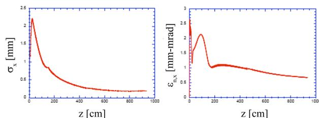
Figure 2: (left) The evolution of RMS transverse beam size  $\sigma_x$  for emittance compensation case, from PARMELA simulation. (right) Evolution of RMS normalized emittance  $\epsilon_{n,x}$  for emittance compensation case.
