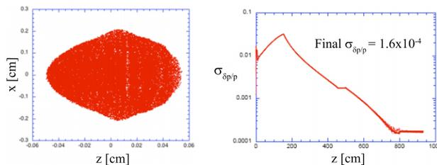
Figure 1: (left) PARMELA simulation results of electron bunch  $(x, z)$  distribution 133 cm from cathode (6.3 MeV energy), showing ellipsoidal beam boundary. (right) Evolution of  $\sigma_{\delta p/p}$  in  $z$  for emittance compensation case, from PARMELA simulation.
