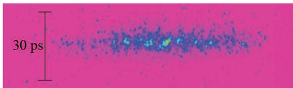
Figure 3: Streak image from SPARC experiment, after correction.
