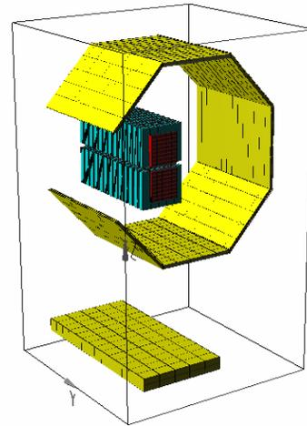
Figure 1: A  $\mu$ -metal shield model used for the calculation.
