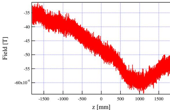
Figure 3: Earth's field distribution measured in MM1.
