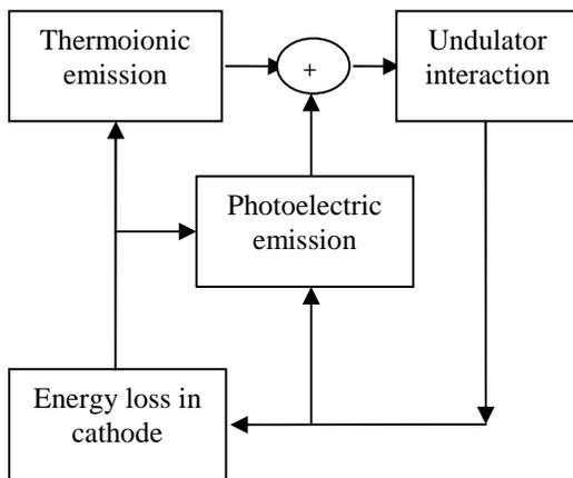
Fig. 1: Block diagram of “hybrid FEL oscillator”.
