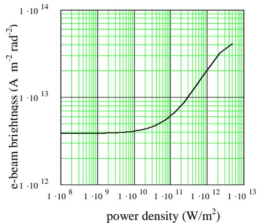
Fig. 4: e-beam brightness [A m<sup>-2</sup> rad<sup>-2</sup>] vs. power density [W m<sup>-2</sup>]
