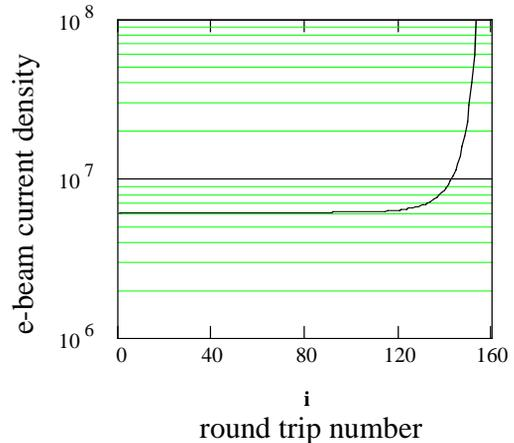
Fig. 6: E-beam current density [ $\text{A m}^{-2}$ ] vs. round trip number.
