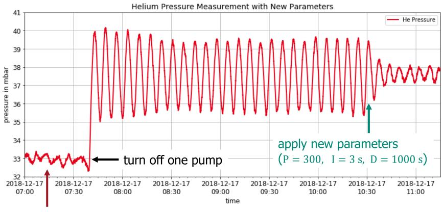
He-level very low, three pumps run at idle (old parameters: P = 250, I = 3 s, D = 0 s)
