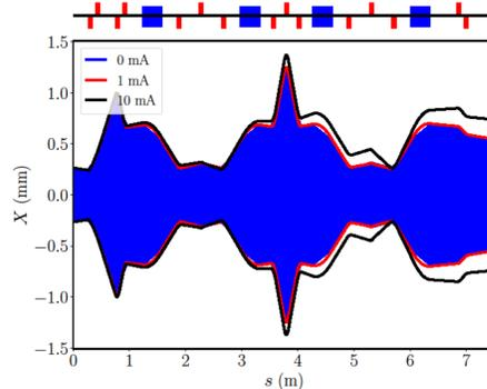
Fig. 1: Evolution of horizontal beam envelope along MARCO at different currents.
