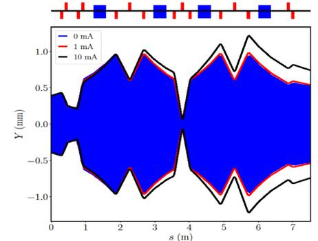
Fig. 2: Evolution of vertical beam envelopes along the MARCO at different currents.
