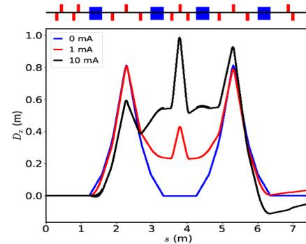
Fig. 3: Evolution of horizontal dispersion  $D_x$  along the MARCO at different currents. Space charge modified dispersion makes the lattice non-achromatic.
