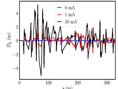
Fig. 4: Evolution of vertical dispersion  $D_y$  along the MESA beamline with space charge at different currents.
