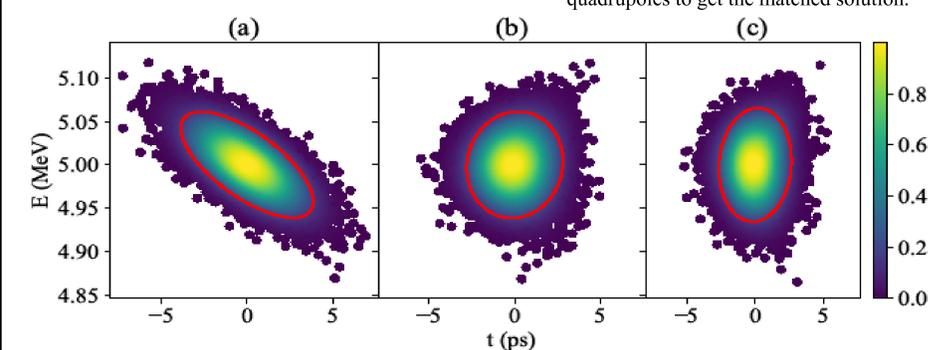
Fig. 5: Longitudinal phase spaces at (a) the start of MARCO, (b) the end of MARCO for  $I = 1$  mA of current, and (c) at the end of MARCO for  $I = 10$  mA. The red ellipses indicate the rms beam ellipse from beam matrix tracking. MARCO works as a bunch compressor even at 10 mA when lattice is matched with space charge.
