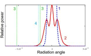
Figure 10: Angular power distribution: electron bunches achromatic bended before third undulator.
