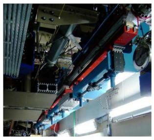
Figure 4: Undulators of the third FEL (7 on the Fig. 3).
