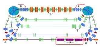
Figure 3: Scheme of NovoFEL installed on a four-track ERL:1- electron injector, 2 - NRF cavities, 3 - round dipole magnet, 4 - rectangular magnets, 5 - quadrupole lenses with dipole correctors, 6 - quadrupole lenses, 7 - undulators of the electron outcoupling system, 8 - mirrors of the optical cavity, 9 - electron dump.
