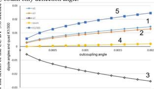
Figure 7: Achromatic bends parameters for the different outcoupling angles: 1,2 - dipole corrector's angles, 3 - angle of the shifted quadrupole, 4 - total angle,  $5 - K_1$  parameter of the quadrupole.
