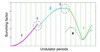
Figure 11: Bunching factor in the undulators system: 1 -first undulator, 2 –second undulator, 3 – bunching factor in the third undulator, calculated along the electron beam propagation axis, 4 – bunching factor, calculated along the optical axis by Genesis code, 5 – drift between 1-st and 2-d undulators, 6 – achromatic bend between 2-d  $\mu$  3-d undulators.
