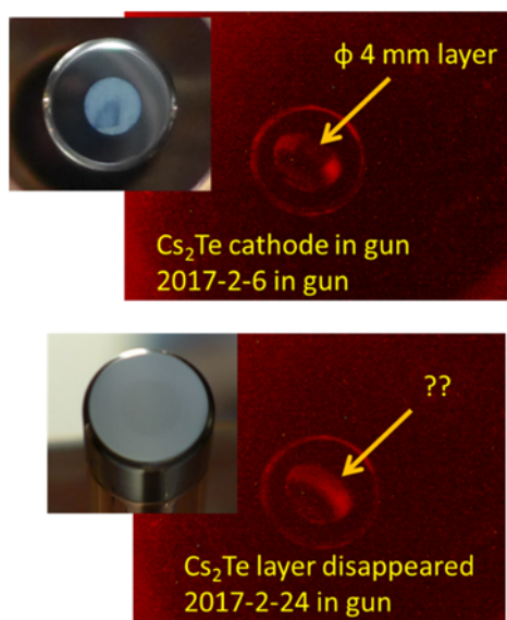
Figure 7: One Cs 2 Te cathode lost film in the SRF gun-II due to overheating. Top: the Mo plug with Cs 2 Te layer in center. Bottom: the layer disappeared in the gun and lost photoemission.
