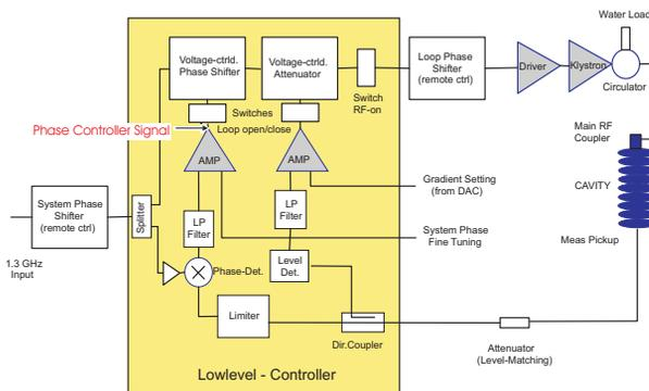
Figure 5: Block diagram of the Low Level RF Controller.
