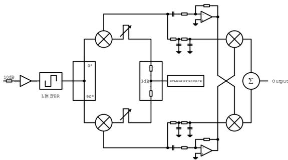
Figure 8: Circuit of the used Resonance-Monitor.
