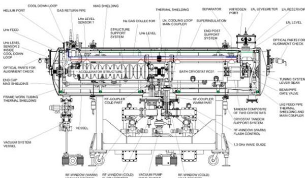
Figure 3: Inner construction of the ELBE cryogenic module.
