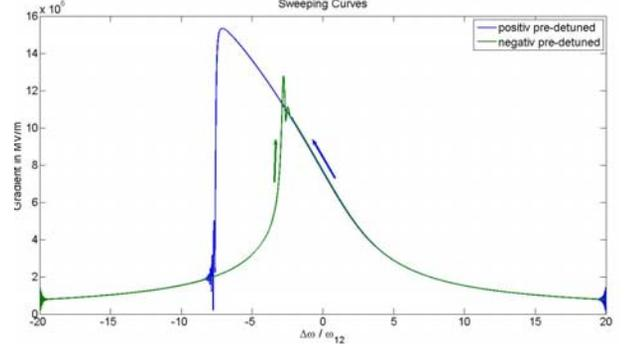
Figure 7: Sweeping curves in single cavity.
