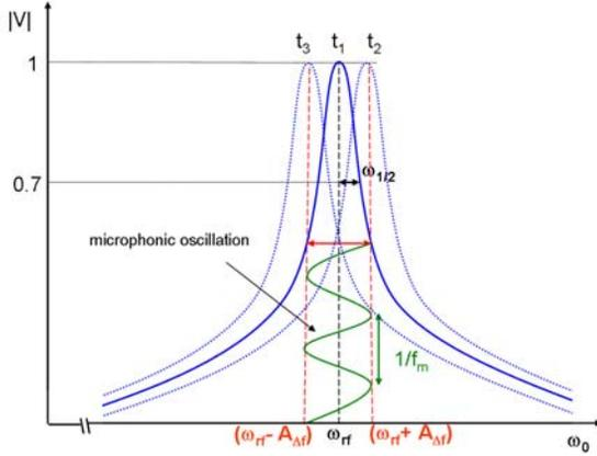
Figure 1: Resonance curve displacement due to microphonic vibrations.
