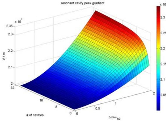
Figure 4: Gradient imbalance as function of  $A_{\Delta f}$  and  $N, f_m = 100$  Hz
