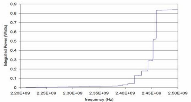
Figure 4. The Power measured at HOM2 integrated from 2.2GHz to the frequency given in the x-axis
